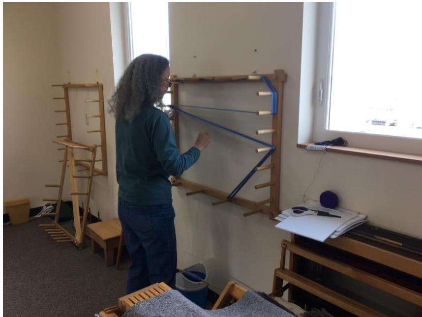
Warping the linen – wall mounted warping board
